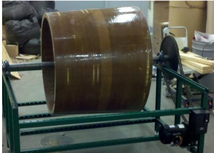
Figure 27: Setup of winding machine
