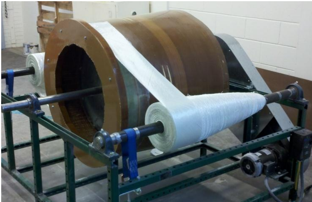
Figure 29: Start of fabric winding
