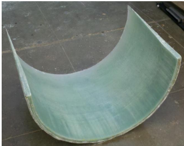
Figure 32: Prototype Root Preform
